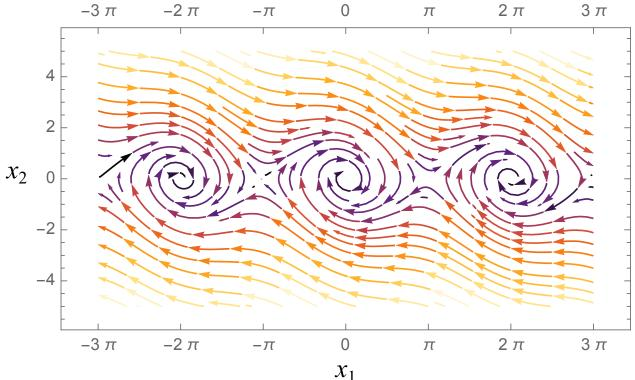
• Phase plane of the damped pendulum,  $b=1/\sqrt{10}$
